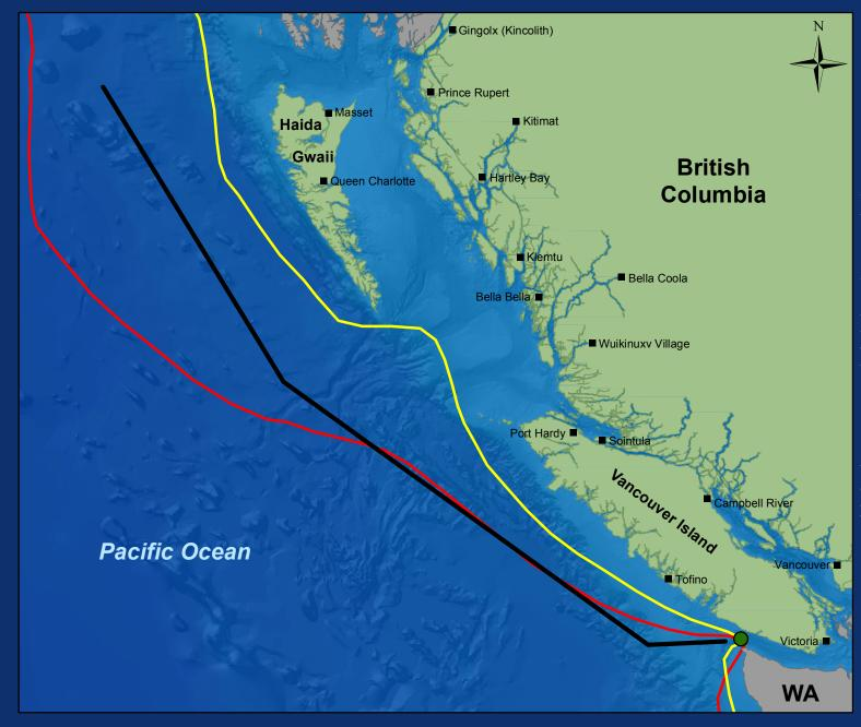
Voluntary Tanker Exclusion Zone Boundary The red and yellow lines indicate the distance a disabled tanker must be from shore in order to be rescued by an available tug before hitting land in different weather conditions. Tankers outside these lines are likely to be rescued before drifting to shore. The black line indicates the Voluntary Exclusion Zone which
